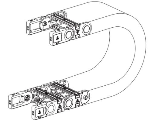
Should be attached to the both ends of the cable carrier.
