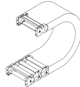
Should be attached to the both ends of the cable carrier
